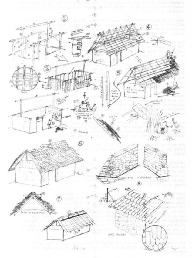
The daubing should be done over a period of several days or weeks, ideally to allow the lower parts to dry out a bit, so that it does not slump or fall out. It can be covered with plastic sheeting etc. to protect it from the weather. When the entire wall is covered with daub, allow it to dry partially and then give the inside and outside another coat, smoothing it well off with the hands. If this is done at a later period, one must wet the existing wall somewhat to give the new daub a grip.
