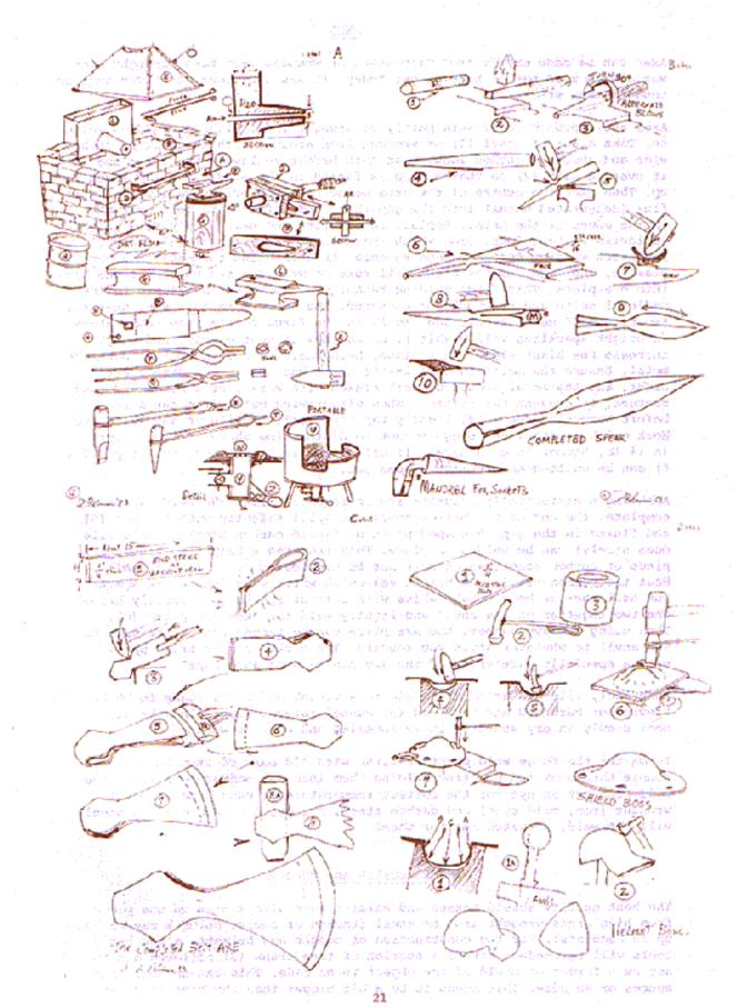
Axes can be made easily from mild steel or wrought iron bars. Wrought iron was always used but is hard to get today. It has a fibrous structure that is tougher than steel.
